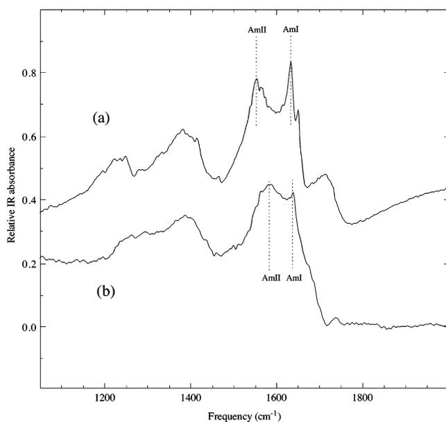
**Figure 6.** FTIR spectra of (a) nanotubes self-assembled from the peptide monomers without the organic Au salts, and (b) nano-doughnuts self-assembled from the peptide monomers in the presence of organic Au salts. AmI and AmII correspond to amide I and amide II, respectively.
