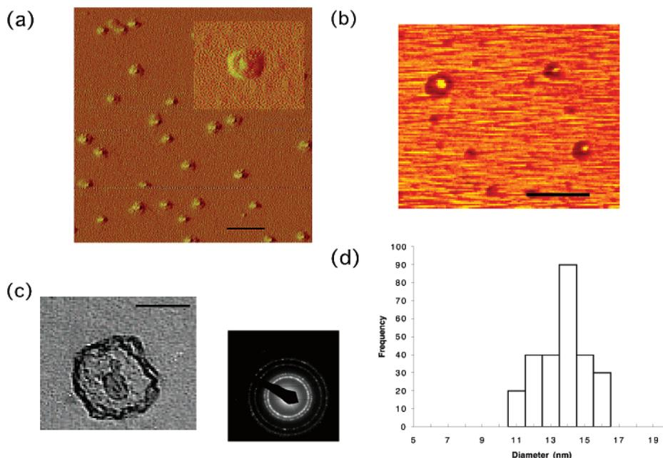
**Figure 3.** (a) SFM topographic image of the peptide nano-doughnuts with Au nanocrystals inside the cavities. Scale bar = 200 nm (inset: The magnified SFM image of the peptide nano-doughnut). (b) SFM phase image of (a). Scale bar = 100 nm. (c) TEM image (left) and electron diffraction (right) of the peptide nano-doughnut–Au nanocrystal complex. Scale bar = 50 nm. (d) The size distributions of the Au nanocrystals grown in the nano-doughnut cavities from the SFM images.
