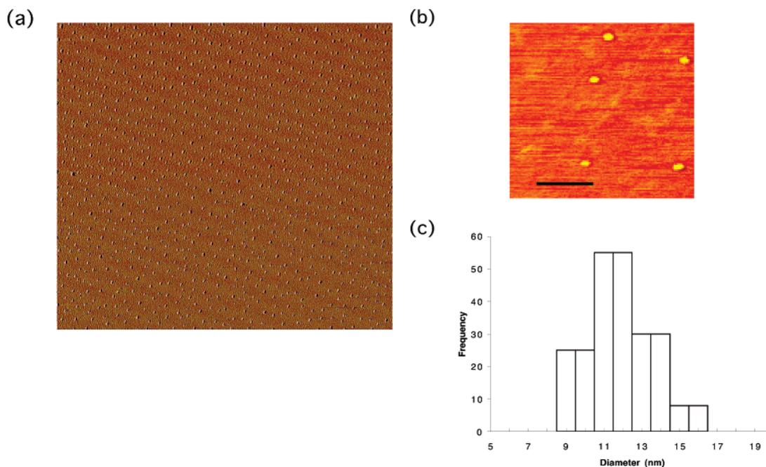
**Figure 4.** (a) SFM topographic image of Au nanocrystals after they were released from the peptide nano-doughnuts via longer UV irradiation (>10 h). Scale bar = 150 nm. (b) SFM phase image of (a). Scale bar = 100 nm. (c) The size distributions of the Au nanocrystals from the SFM images.
