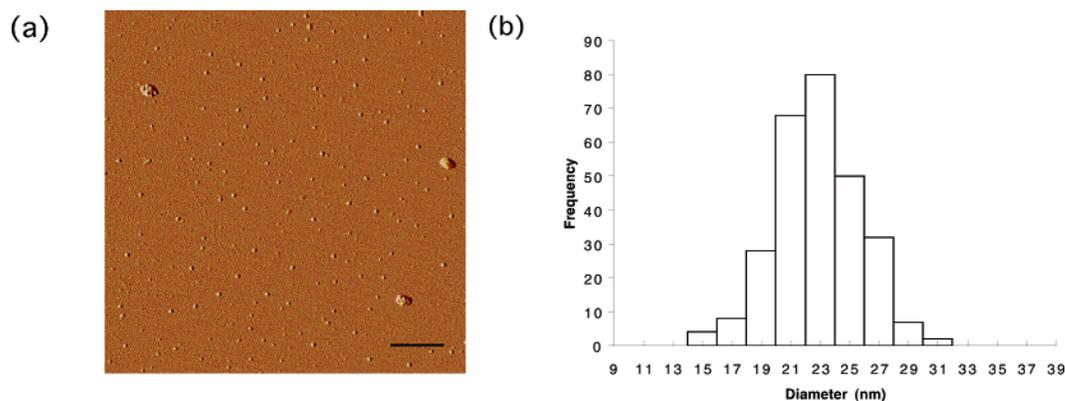
**Figure 5.** (a) SFM topographic image of Au nanocrystals after reducing the peptide nano-doughnuts by hydrazine hydrate. Scale bar = 150 nm. (b) The size distributions of the Au nanocrystals from the SFM images.
